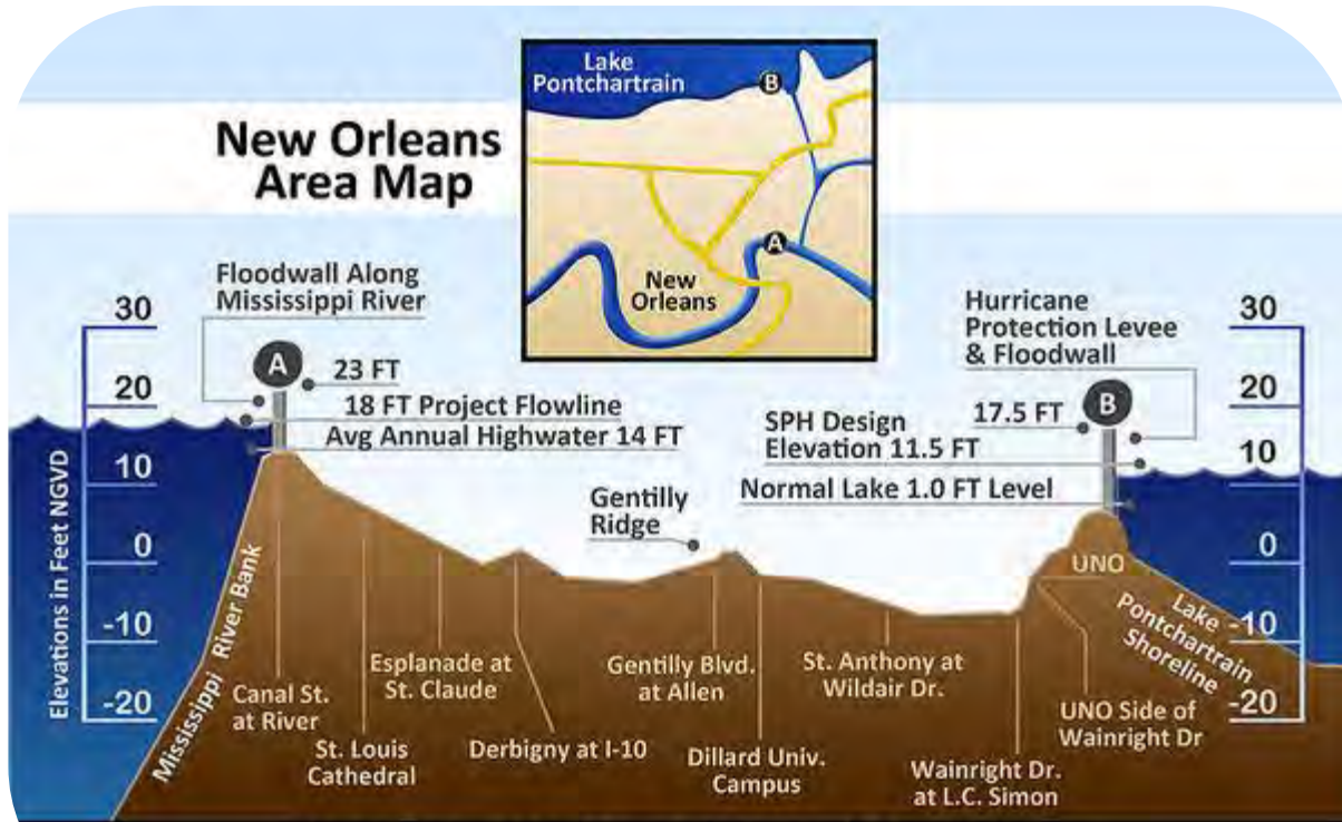
City of New Orleans Ground Elevations From Canal St. at the Mississippi River to the Lakefront at U.N.O.
