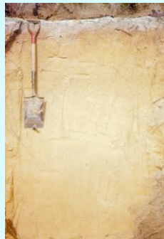
Candler (HSG "A") soil profile, SHGW > 6 feet B.L.S.
