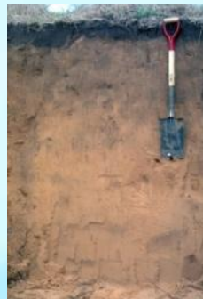
Tavares (HSG = "A") soil profile, SHGWT 42" to 72" B.L.S.
