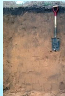
Tavares (HSG = "A") soil profile, SHGW 42" to 72" B.L.S.
