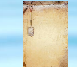
Candler (HSG "A") soil profile, SHGWT > 6 feet B.L.S.
