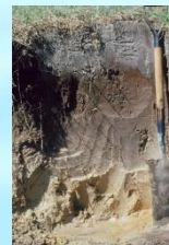
Narcoossee (HSG = "C") soil profile, SHGWT 18" to 42" B.L.S.
