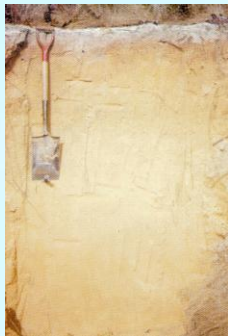
Candler (HSG "A") soil profile, SHGWT > 6 feet B.L.S.
