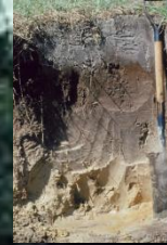
Narcoossee (HSG = “C”) soil profile, SHGWT 18” to 42” B.L.S.
