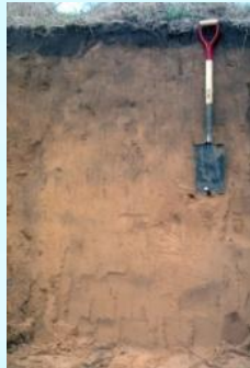
Tavares (HSG = "A") soil profile, SHGWT to 72" B.L.S.
