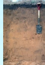
Tavares (HSG = "A") soil profile, SHGWT 42" to 72" B.L.S.
