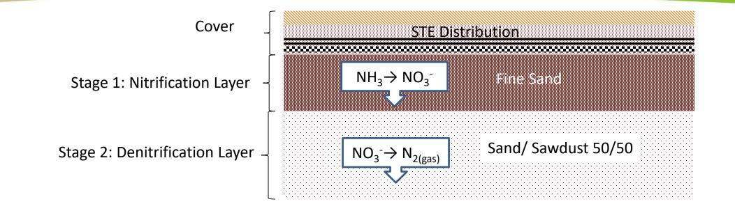
Underlain by impermeable liner for effluent collection or media with high water retention capacity (permeable layer)
