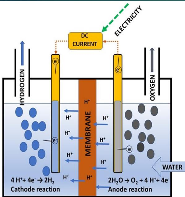
Low temperature membrane electrolyzer splitting water
