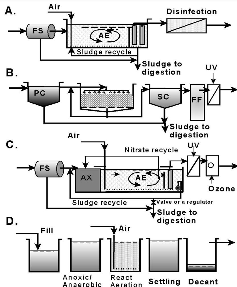
Membrane Filter AX - Anoxic, AE - Aeration, FS-Fine screens, PC-Primary Clarifier, SC-Secondary clarifier, FF-Fine filtration
