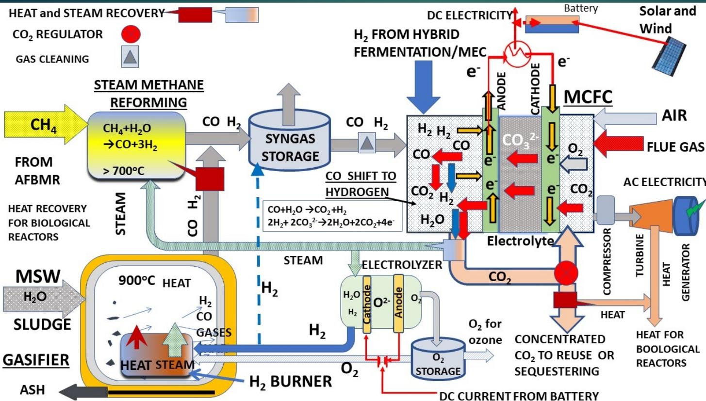
ANova DC produces electricity, clean steam (water), concentrated sequester able CO<sub>2</sub>, heat energy and pure oxygen that has a commercial value.
