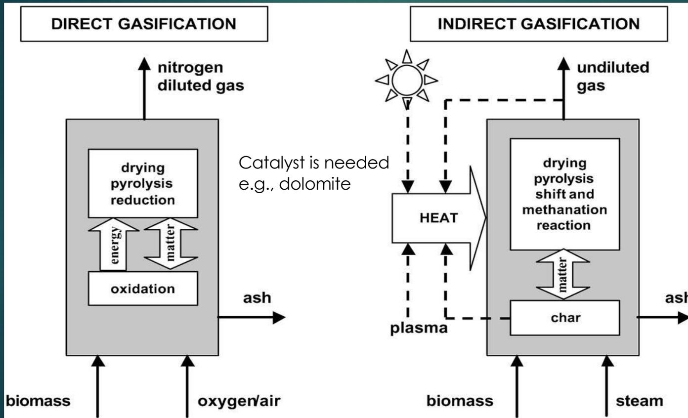
A chemical high temperature decomposition of organic matter into synthetic biogas (syngas), char and tar, and biofuel.
