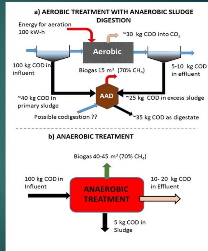
Comparison of aerobic and anaerobic treatment
