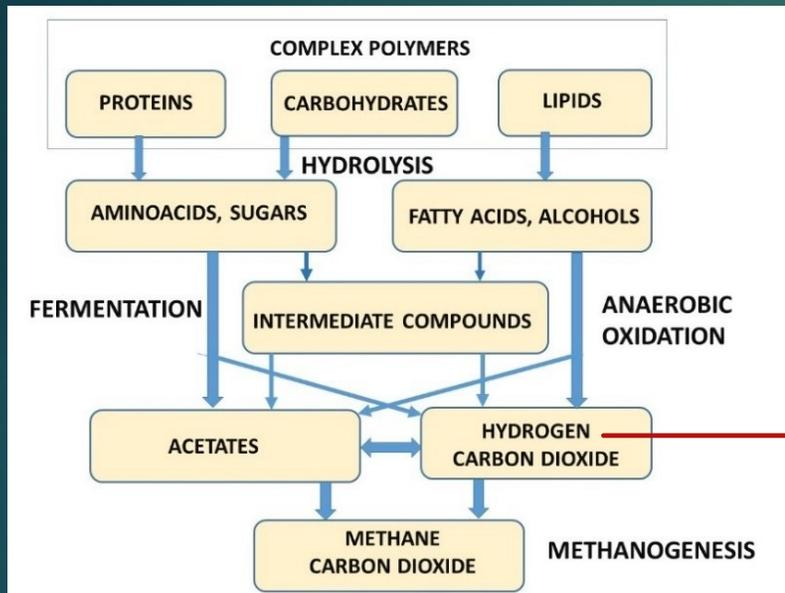
If H<sub>2</sub> is desired digestion product, methanogenesis is suppressed by keeping pH at 5.5
