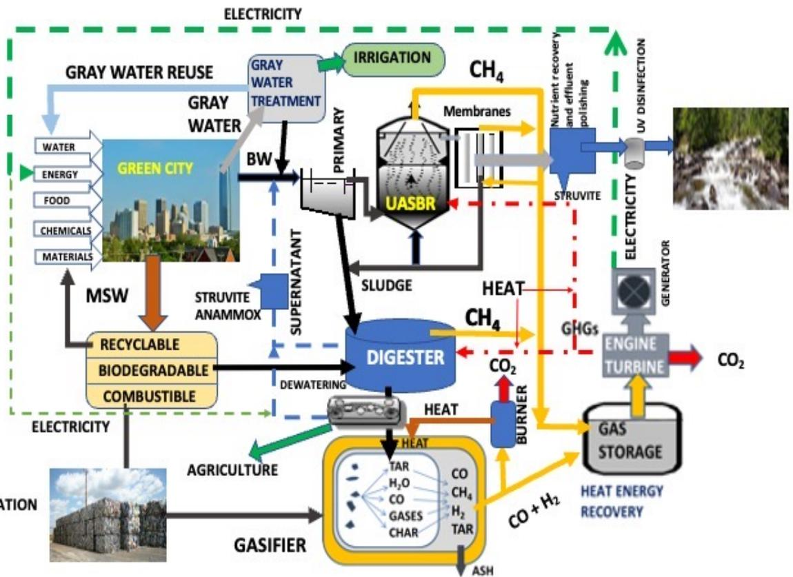
Implementing water conservation and grey water recovery increases COD concentration in used water that requires biogas producing anaerobic treatment.
