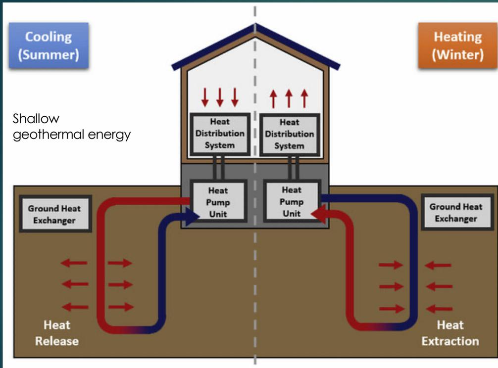
Heat pumps can be used to extract heat and cooling from sewers, lakes, ground, air, etc., with 80% energy conversion efficiency
