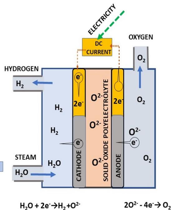
High temperature SOFC working in reverse to make H<sub>2</sub> and O<sub>2</sub> from steam
