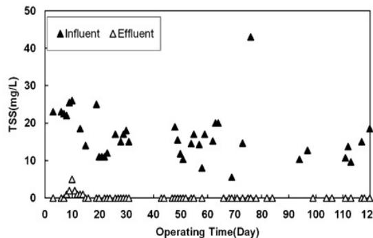
FIGURE 6. Removal behavior of SCOD and TSS in the AFMBR component of the two-stage AFBR/AFMBR system at a permeate flux of 10 L/m<sup>2</sup>/h.
