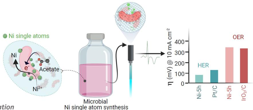
➤ Total overpotential for Ni-SA was 410 mV compared to 440 mV (Pt/C and IrO<sub>2</sub>)
