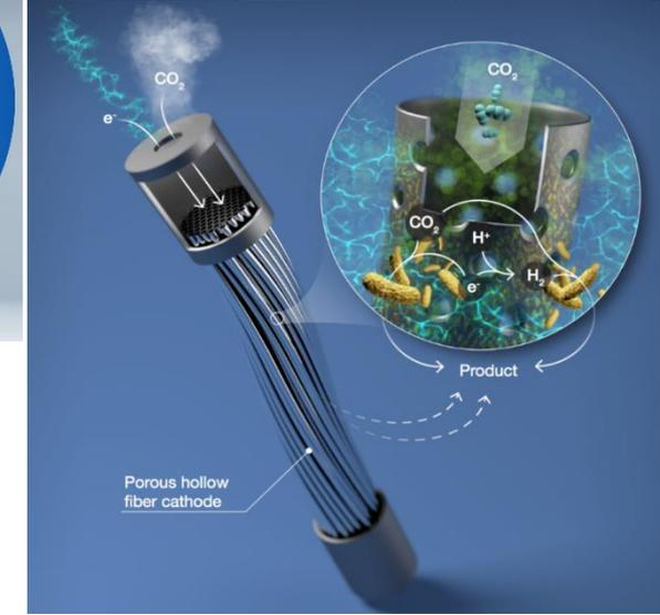
**Conversion of CO<sub>2</sub> to CH<sub>4</sub> with high Faradaic efficiency (> 80%) compared to 3% through gas-bubbling in electrolyte**
