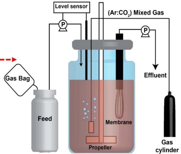
➤ **Stable reactor performance with NRR of  $0.27 \pm 0.01$  kg-N m<sup>-3</sup> d<sup>-1</sup> and ~92% N-removal efficiency**
