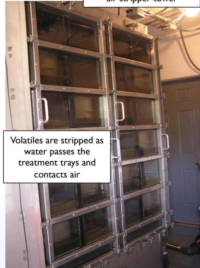
Volatiles are stripped as water passes the treatment trays and contacts air
