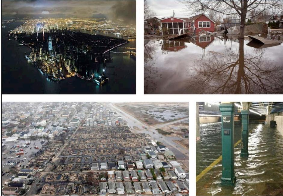
Fire in Breezy Point – more than 100 homes completely destroyed. Flooding limited firefighter access; damage to private water main network forced firefighters to pump seawater to fight fire.
