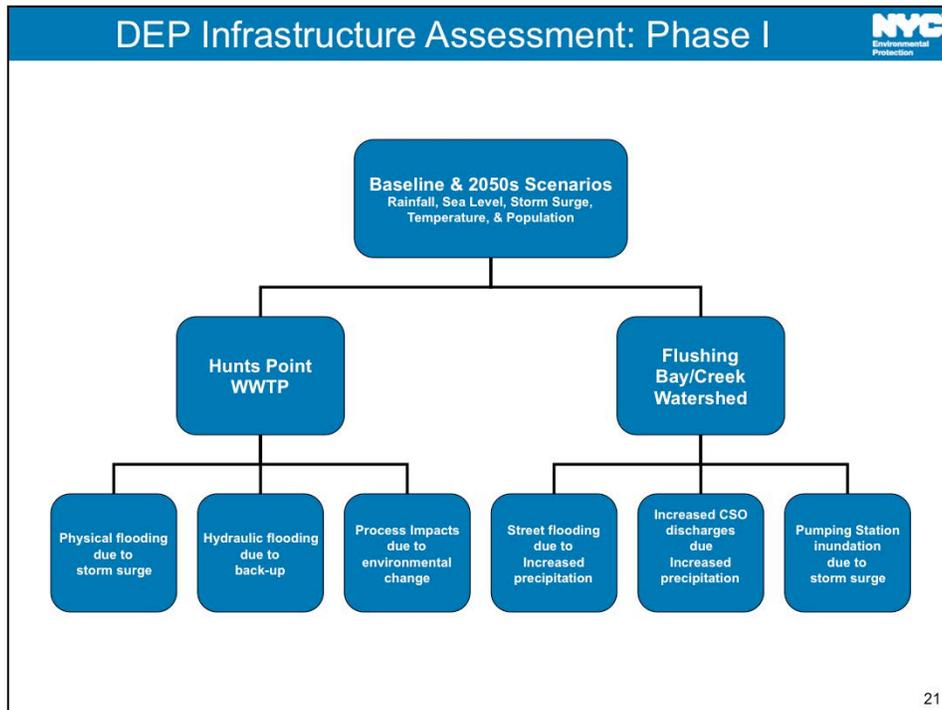
The DEP performed a vulnerability assessment for one wastewater treatment plant, 8 pumping stations and a 16,377 acre drainage area.
