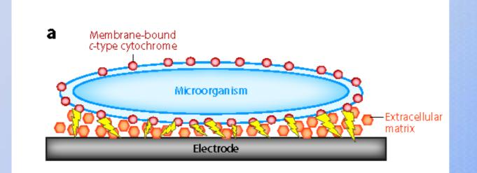
Short-range electron transfer through redox active proteins such as c-type cytochromes (associated with outer cell surface)
