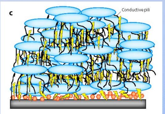
Long-range transfer through pili – a conductive bilofilm with "nanowires"
