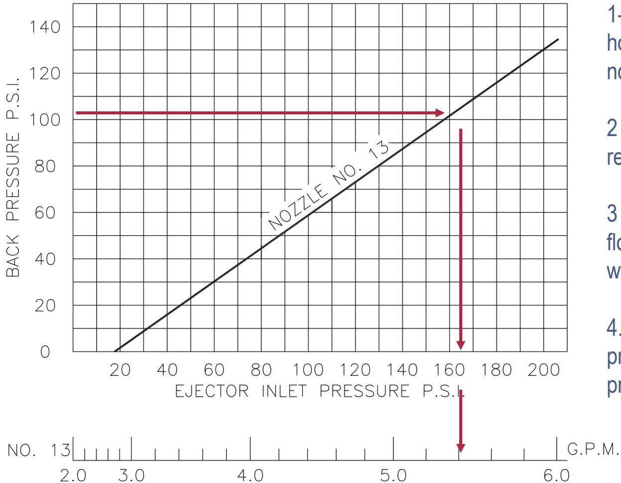
1- Start with back pressure, follow horizontally to the intersection of nozzle curve
