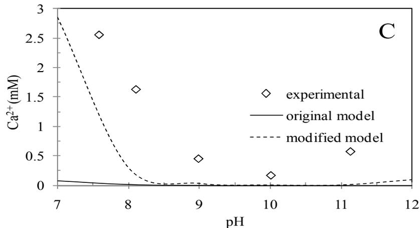
**Modified model** - only struvite and calcite precipitates were allowed to precipitate
