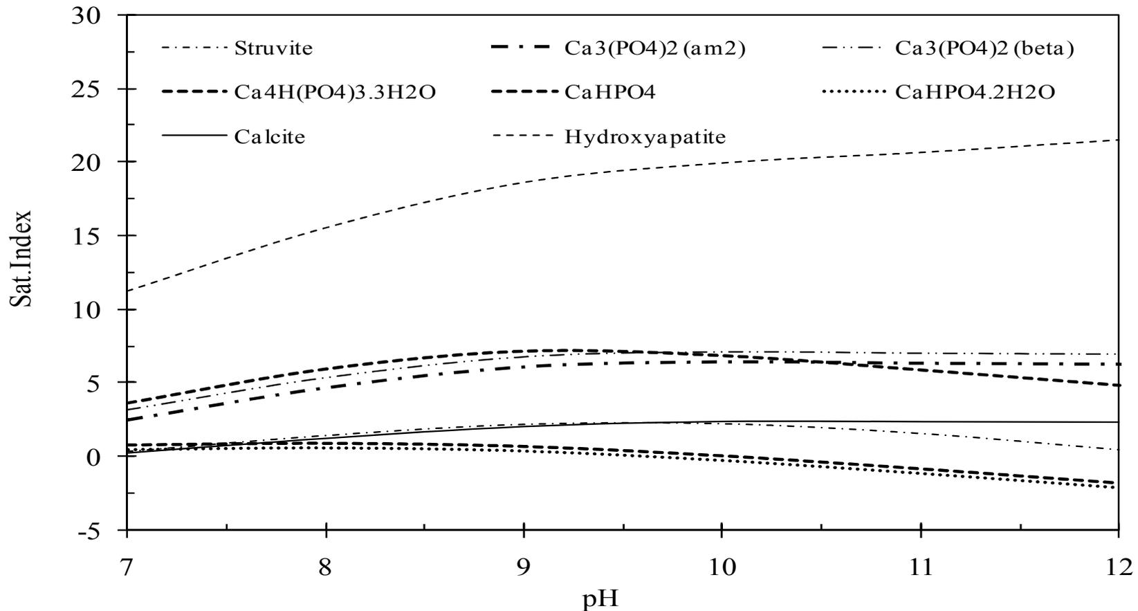
Chemical equilibrium model prediction of saturation index of phosphate precipitates as a function of pH for effluent water treated with 0.3 g/L of DL
