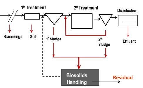
Extending biological treatment to include bulk carbon, nutrient, pathogen AND TOrC reduction/removal can help reduce overall energy requirements for WRRFs of the future
