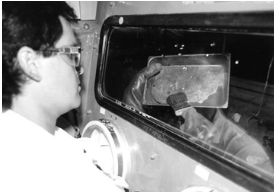
An operator brushes oxide from a plutonium button. The plutonium button was the raw material shipped from the Department of Energy's Hanford or Savannah River sites.
