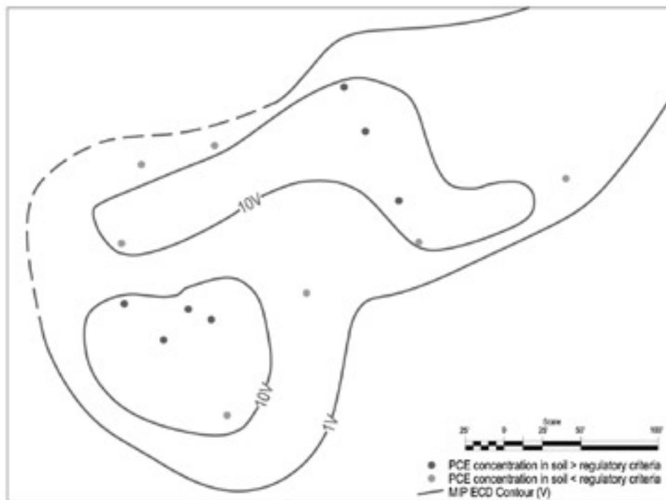
FIGURE 4. Site 1: plan view figure showing MIP ECD contours and soil boring PCE results (regulatory criteria = 1,000 ug/kg).
