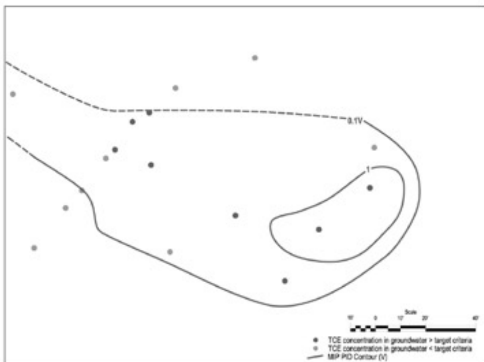
FIGURE 6. Site 2: plan view figure showing MIP PID contours and groundwater TCE results (target criteria = 1,000 ug/L).
