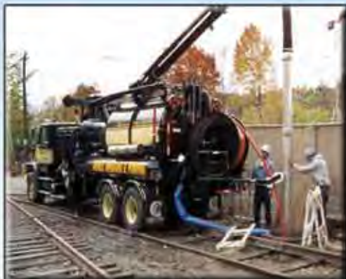
SEWER CLEANING: High-Pressure Jetting / Power Bucketting: Single and double-pump, jet-vac combination units with line jetting capabilities of 175 gpm / 2,500 psi literally scour sewers clean. Specifically sized buckets quickly and thoroughly remove all debris from severely clogged sewer lines.
