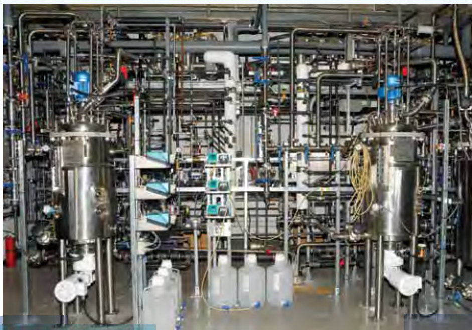
Top: Trichoderma-biocontrol agent; right: Pilot plant with 15L, 150L and 2000L fermentors for bioconversion of wastewater and wastewater sludge to value added products.
