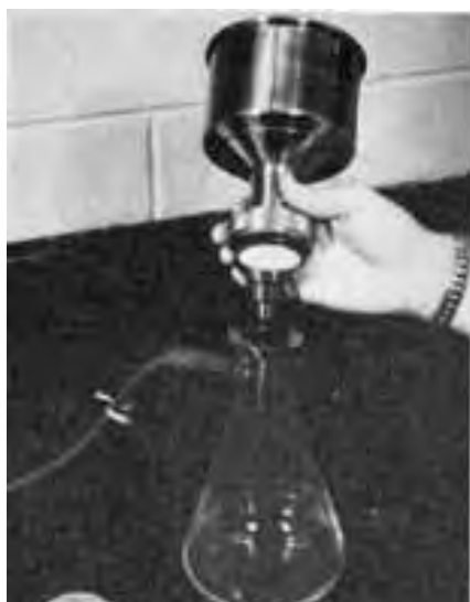
Figure 6 Membrane Filtration of Water Samples
