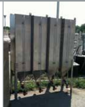
Algal dewatering unit designed by Dr. Belinda Sturm and Stacey Lamer, Bartlett & West, Inc. and constructed by CDI Contractors, Kansas City, Kansas.
