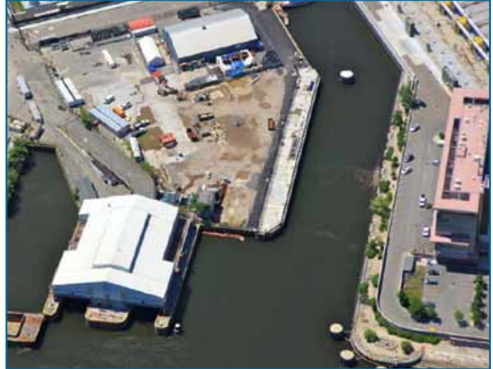
Construction of a new 360 ft long dock and dredging of the canal provides a safe harbor for NYCDEP research and waterway skimming vessels, protecting them from high waves and powerful storms. Locating the new sludge dock adjacent to and across from the Newtown Creek Nature Walk enables the local community to observe and appreciate the civic value of a modern wastewater treatment plant.
