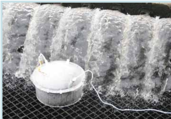
Obtaining a Foul Air Sample with a Flux Chamber on a Tricking Filter
